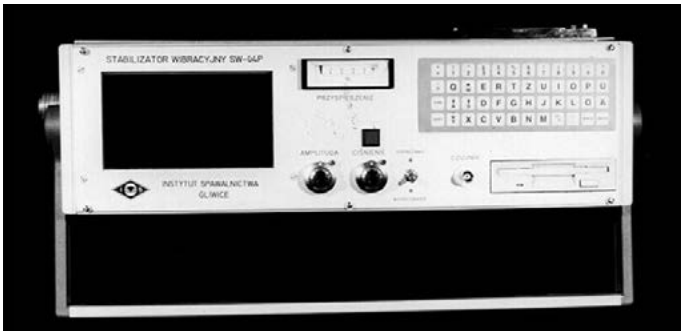
Fig. 5. Control panel of the SW04P stabiliser
